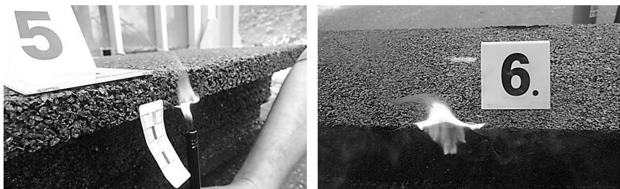
**Figure 5.** Test 3 – small fire attack.
